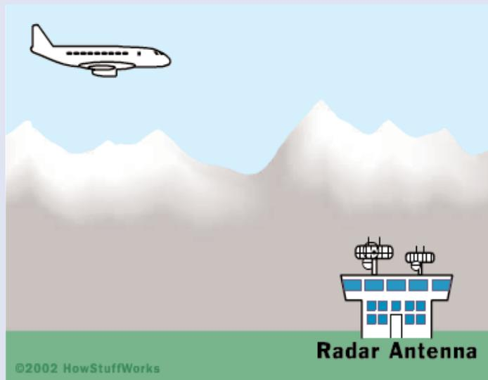
*The radar antenna sends out a short, high-power pulse of radio waves at a known frequency. When the waves hit an object, they echo off of it and the speed of the object Doppler-shifts the echo. The same antenna is used to receive the much-weaker signals that return.*
