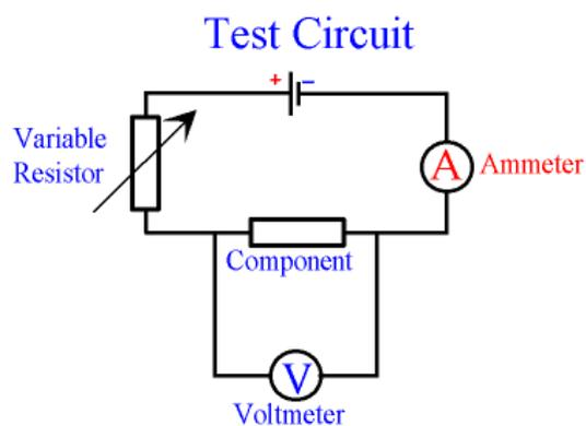
2. Set up the circuit as shown and note the current (I) and potential difference (V)
