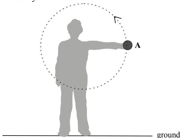
A student swings a ball in a circle of radius 70 cm in the vertical plane as shown. The angular velocity of the ball is  $10 \text{ rad s}^{-1}$ .
