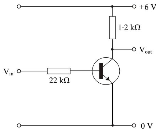
The circuit diagram represents a voltage inverter.
