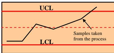
(i) Outline the role of the *upper control limit* (UCL) and the *lower control limit* (LCL) lines on the graph shown.
