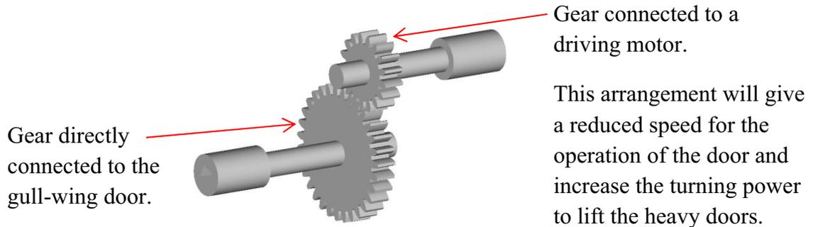
The motor can be controlled by switching that allows the motor to reverse as well as drive forward, speed control is also feasible. A DPDT switch can be used.
