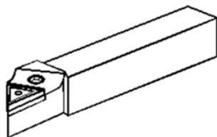
Carbide insert cutting tool
