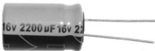
The photograph shows the device **H** used in the circuit. Use the data printed on the device to calculate the maximum energy that it can store. (9)
