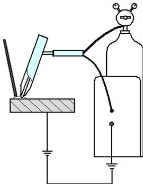
An arc is formed between the non-consumable electrode and the metal being welded. The inert gas shielded arc is used to flux the joint, Argon is often used to prevent oxygen getting to the joint area. A filler metal is added manually to the weld pool when necessary. A high frequency generator provides a path for the welding current.
