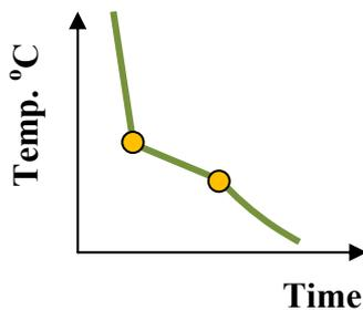
The cooling curve for a combination of metals highlights the start and end of solidification for that particular alloy.
