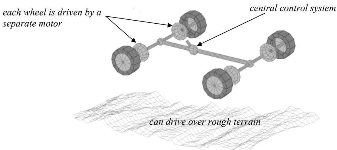
This all terrain surveillance vehicle has the facility to drive each wheel separately as each wheel has a motor control system. These motors are centrally controlled to turn on each motor when required.
