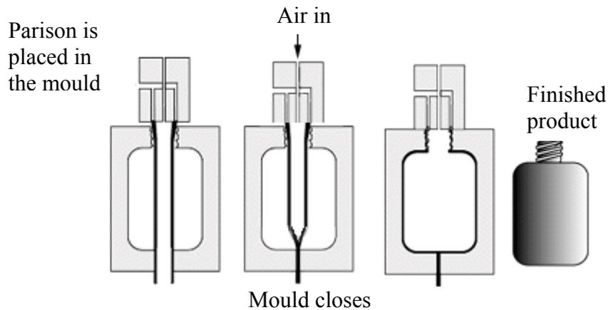
An extruded thick-walled tube, called a parison, is placed in the mould. The mould closes and air is blown into the parison. The parison takes the shape of the mould.
