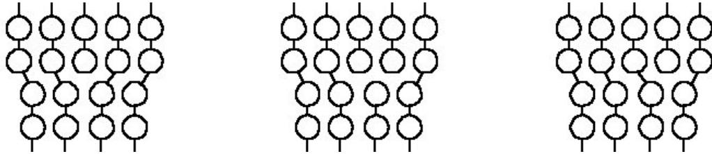
As the shear force is exerted, the fault moves to the next line and may move to the grain boundary. Slip in metals is largely due to the presence of dislocations and will influence material properties.
