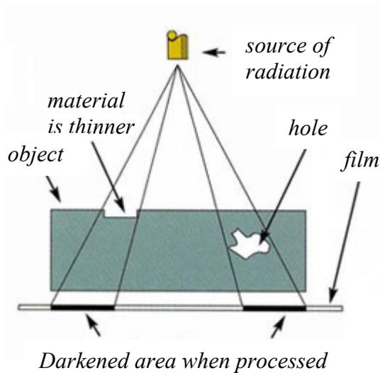
Radiation from an x-ray tube is passed through the weld. If no defects are present, the amount of absorption is uniform across the area exposed to the x-ray beam. If a defect is present in the weld, a smaller amount of rays is absorbed giving a variation in the intensity of the emergent beam. This can be detected by placing a photographic film on the side of the material opposite the radiation source. On a negative film, the defect shows as a dark spot.
