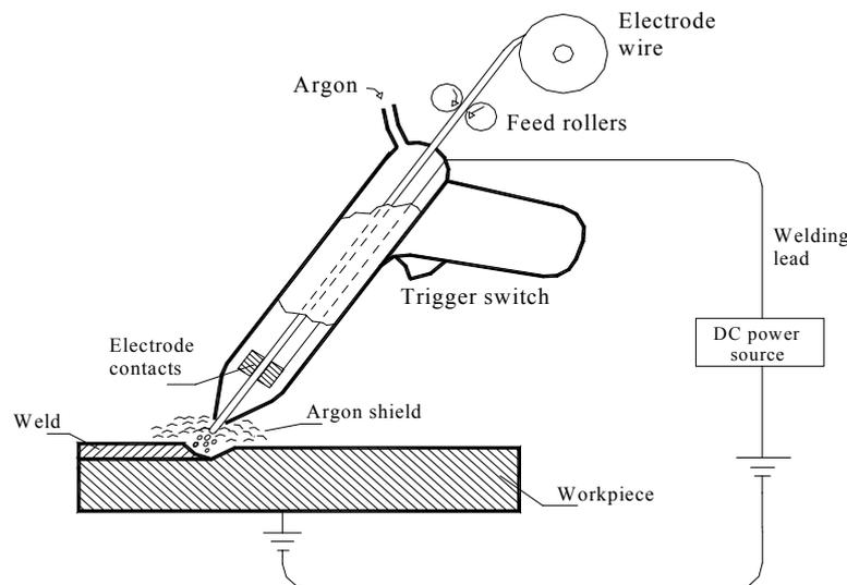
Metal inert gas welding is a semi-automatic process. It operates on principles similar to manual metal arc welding. A consumable bare wire electrode is fed continuously through the welding torch or gun into the weld pool area. Fluxing is
