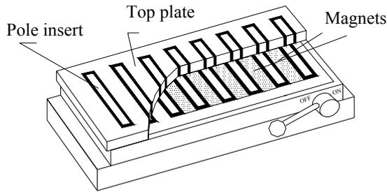
Chuck in the OFF position as the magnets are out of phase with the top plate. The workpiece is now released.
