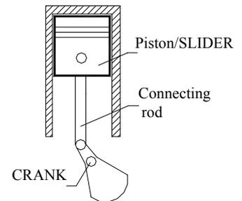
**Function:** A crank and slider mechanism changes rotary to reciprocal motion or vice-versa. **(Operation) 10 (Function) 6**
