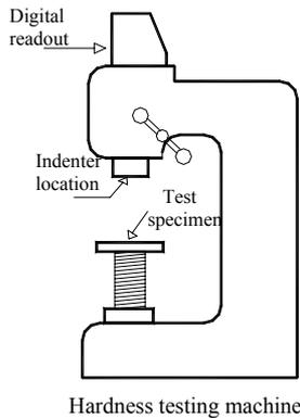
A diamond shaped indenter is forced into the specimen. The diagonal length of the square is measured. This measurement is taken by a special microscope for accuracy. It is then converted into a Vickers hardness number. **8**
