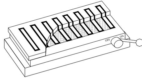
ON position as the magnets have moved in line with the top plate therefore the work is securely held.
