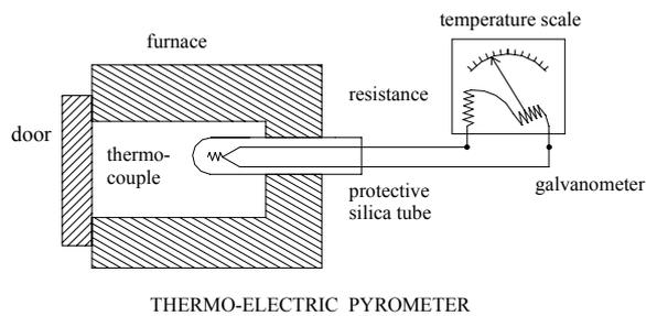
Applications for both would be measuring temperature in heat treatment furnaces.
