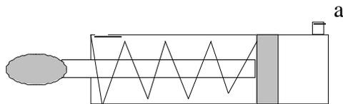
Air entering port a of the cylinder will push the piston
